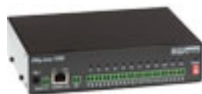
HWg-Juno 1200 12 DI for Dry contacts None DO WEB server Ethernet 100 Mbit PoE (IEEE 802.3af) or 12V wall plug power adaptor Wall mount or rack mount kit
