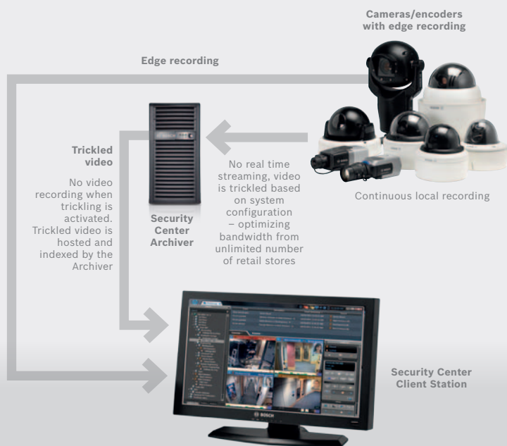
Edge Recording & Video Trickling Architecture
