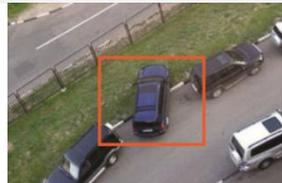
Provides the parking occupancy level and free parking slot availability by detecting vehicle entry and exit by monitoring these transition points in parking lot areas.
