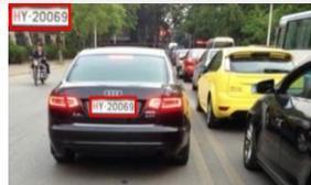
Detects the presence of vehicle license plate (or number plate) and captures the image of the license plate along with the vehicle.
