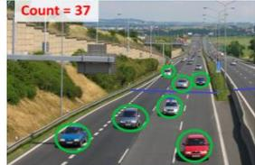
Counting of vehicles that cross a virtual line in a vehicle lane or entry / exit gates.
