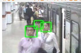
Detects and tracks the human face in the camera view, and also captures the face image and stores it in the database for future reference.
