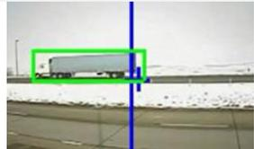
Detects speeding of any vehicle above specified speed limit observed in camera installed parallel to the road.
