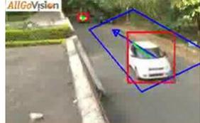
Detects vehicle movement in a direction opposite to user specified direction.
