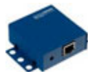
HWg-Juno 101 1 DI for Dry contact 1 DO Relay (50V) WEB server Ethernet 100 Mbit PoE (IEEE 802.3af) or 5V wall plug power adaptor Wall mount
