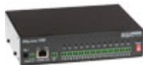
HWg-Juno 1200 12 DI for Dry contacts None DO WEB server Ethernet 100 Mbit PoE (IEEE 802.3af) or 12V wall plug power adaptor Wall mount or rack mount kit
