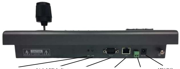
PW LED lights when device is powered on.
